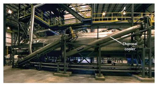
Figure 15. Charcoal cooling system in vacuum pyrolysis plant (Source: Group Pyrovac).
