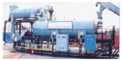
Figure 9. The steam produced by this auger pyrolysis unit with a thermal oxidizer can be used to generate electricity. (Source: <u>http://www.internationaltechcorp.org/IT-info.htm#convert</u>).
