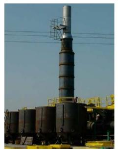
Figure 8. Several batch pyrolysis reactors linked to an after burner known as a CML process (Source: <u>http://www.drveniugljen.hr/assets/files/ prezentacije/06\_Christian\_Bedrossian.pdf</u>).
