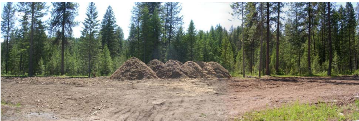
Figure 5: Slash ground into a uniform product ready for transportation to the biomass facility
